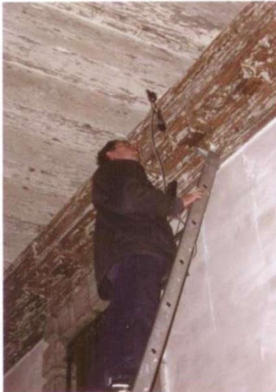
Reading the humidity inside the beam.
